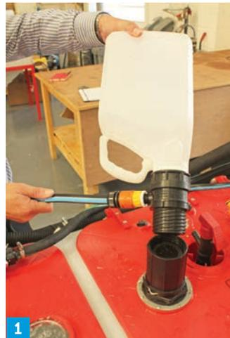
**The Banjo system has a tank adaptor retrofitted to the sprayer**
