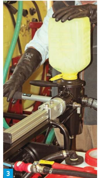
**The EziConnect uses a Venturi valve to suck neat chemical out of the attached container**
