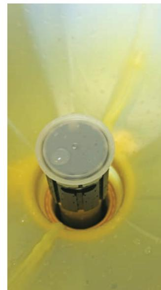
A lever-mounted probe moves up and down to vary chemical flow
