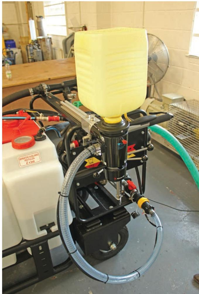
The EziConnect's use of suction and air helps speed up the filling process
